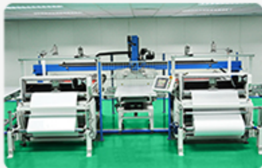
Automatic EVA & Backsheet loading
